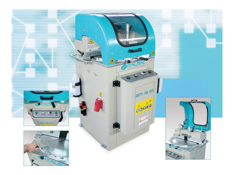
Single head cutting off machine with manual and automatic raising of the blade. Possibility to perform trimming operations.
